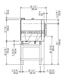
CWII Cold Water inlet 1 CWI2 Cold Water Inlet 2 ΕI Electrical inlet (power) Gas connection
